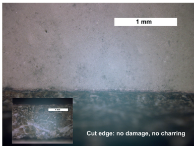
Cutting of Leather 1.3 mm thick Speed: 1.0 m / min
